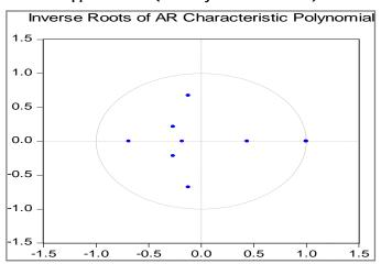
Inverted AR roots are within the unit root circle and signify that model is stable.
